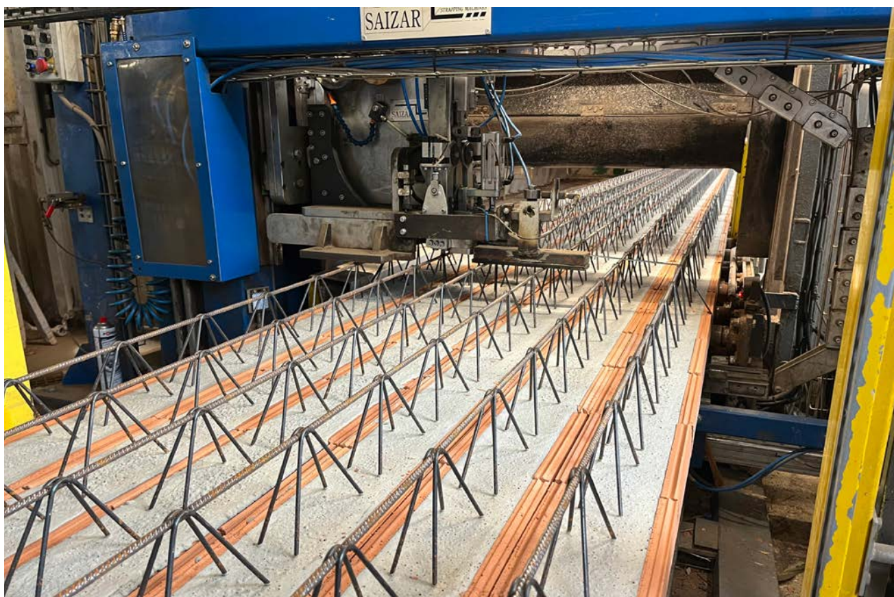
Foto 4: Strapping machine/dispatch of POT floor beams
