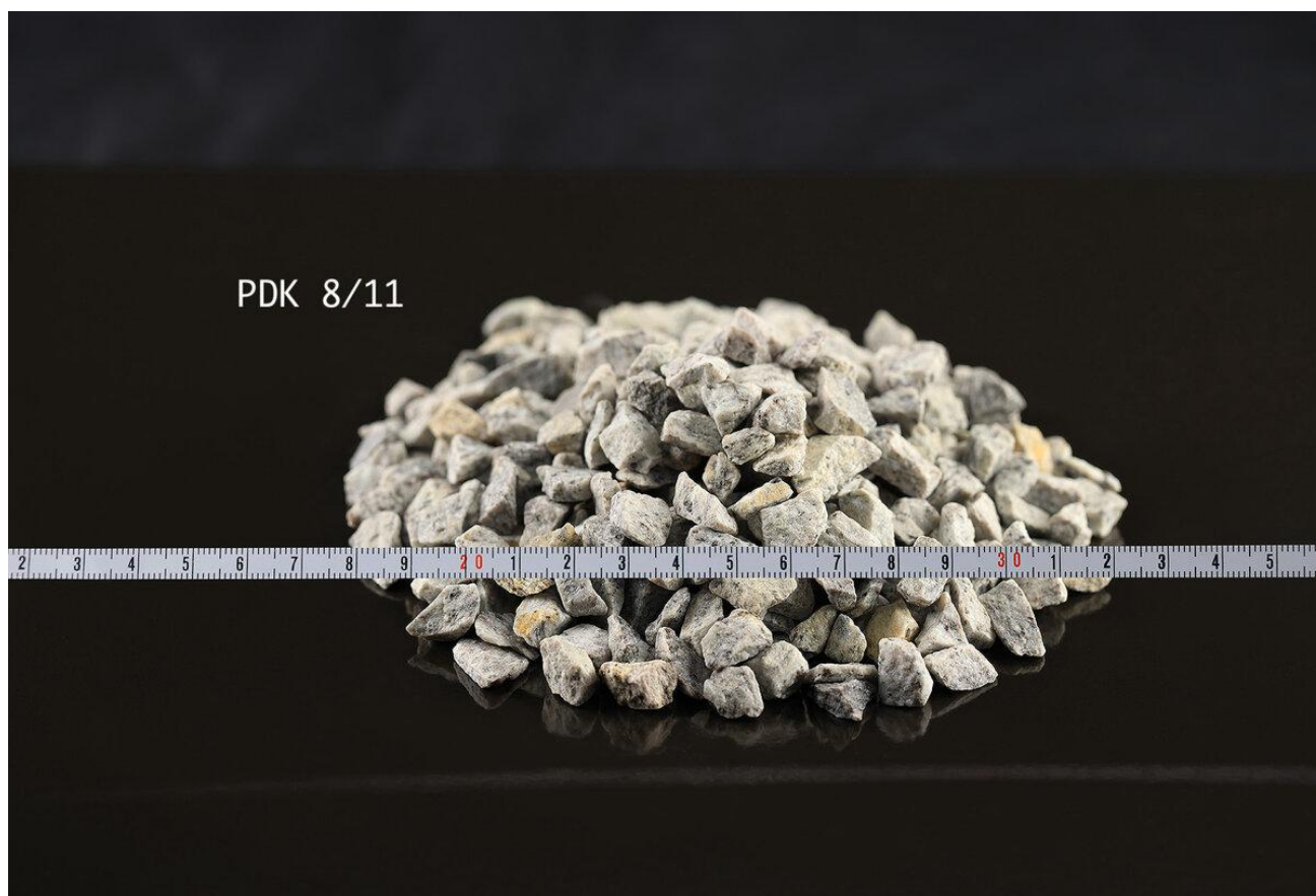
Figure 1 Graded crushed aggregates, PDK 8/11: natural crushed aggregate
