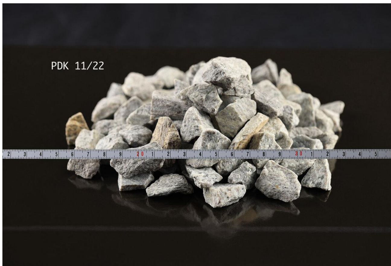
Figure 1 Graded crushed aggregates, PDK 11/22: natural crushed aggregate
