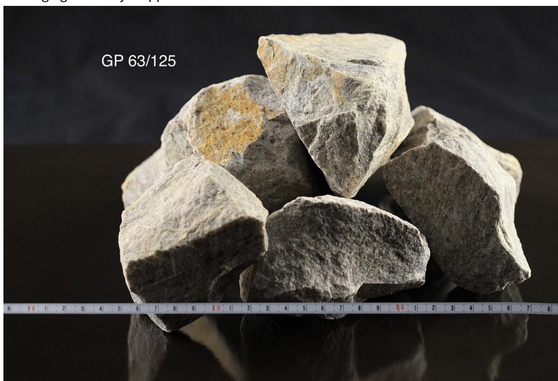
Figure 1 Crushed rock fill, macadam, GP 63/125: gravel, poorly graded
