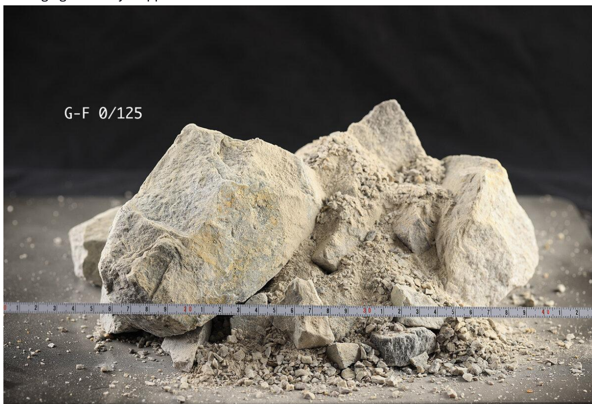
Figure 1 Crushed rock fill, macadam: G-F 0/125: gravel, with an admixture of fine-grained soil
