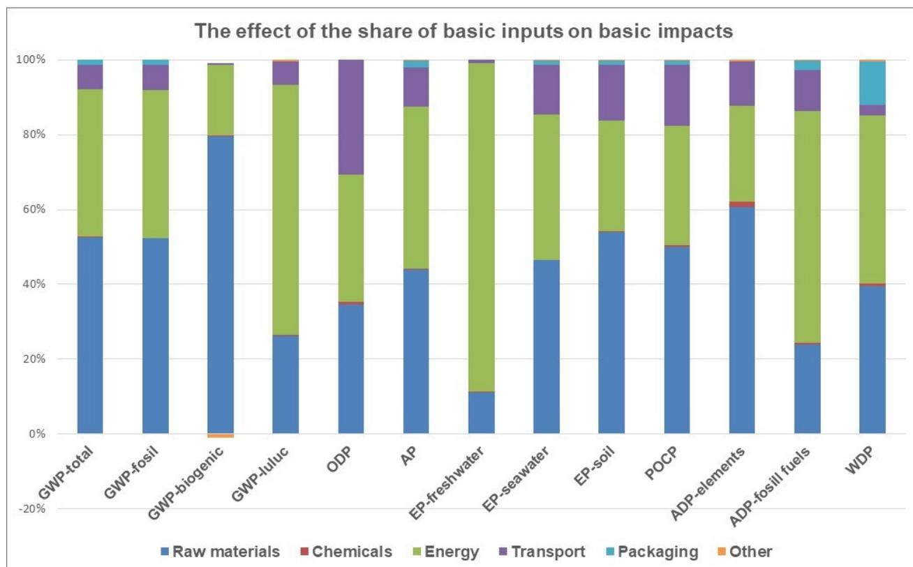
It can be seen from the figure that the **consumption of raw materials (mainly cement)** and **electricity** and its energy mix (CZ) have a very significant influence on environmental impacts. To a lesser extent, the effect of **transport** is also applied.
